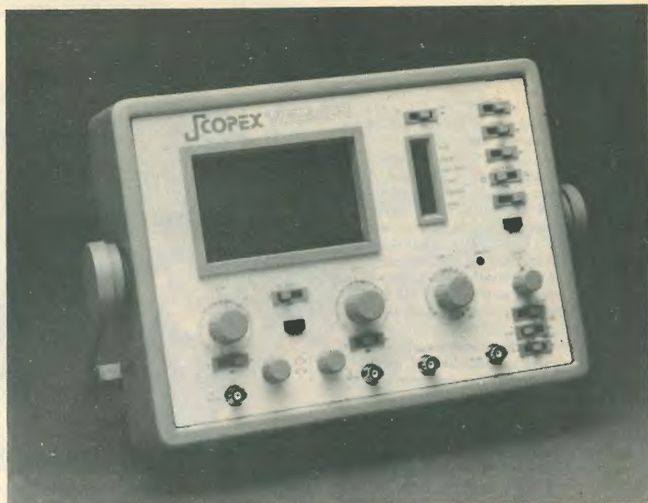
The Scopex Voyager oscilloscope is the first commercially available to include a flat i.c.d., making it smaller and with lower power requirements than conventional instruments.
